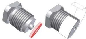
In both cases the torque must be applied using two hexagonal spanners, one on the flat faces of the instrument/process coupling and the other on the pressure connection.
